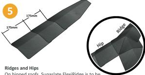
On hipped roofs, Supaslate FlexiRidge is to be installed from the eaves and working up the hip until it meets the ridge. Be sure to maintain an even cover to ensure an even finish at the crown of the roof, we recommend 175mm. Then follow the same method to work along the ridge. The crown can be mitred or dressed with lead.
